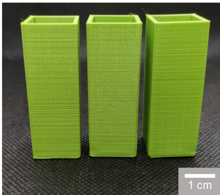
Supplementary Figure 24 | Photographs of the custom-designed photoreactors for solar vapour characterization. 3D-printed reactor with a dimension of 1.5 \times 1.5 \times 5.0 \text{ cm}^3 . The reactors were printed using polylactic acid (PLA) filament.
